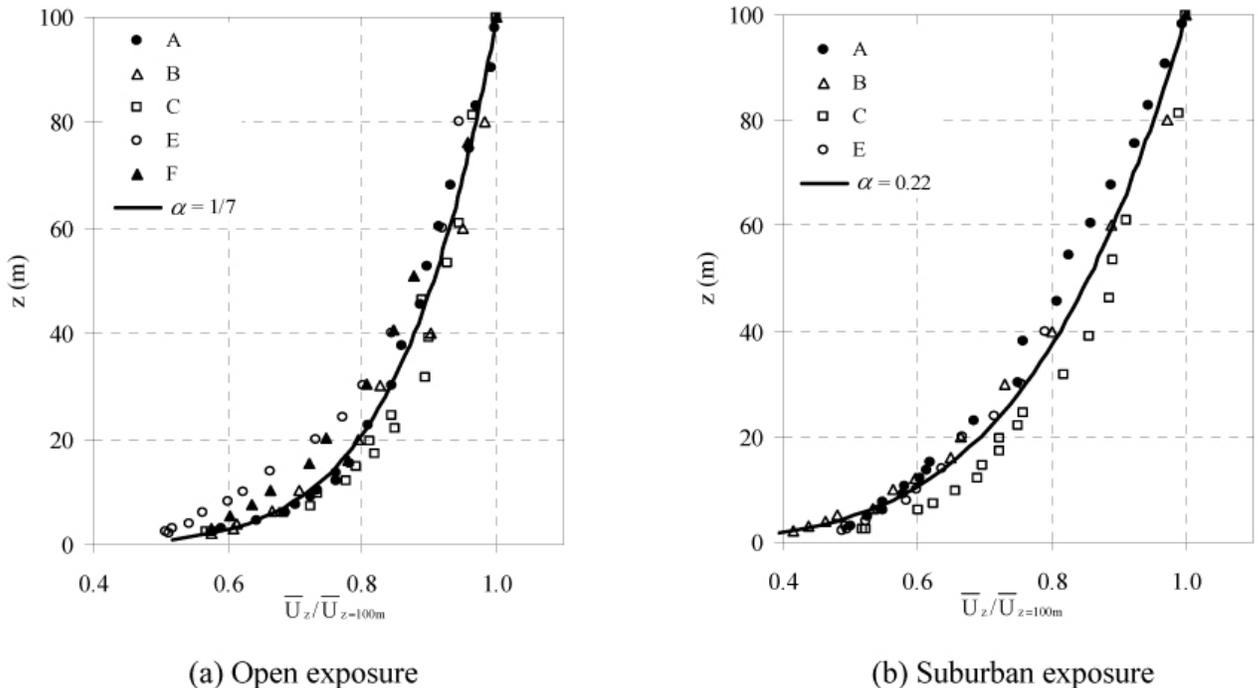
Figure 3.1. Wind speed profiles in simulations by wind tunnels participating in the Fritz et al. (2008) comparison (Bienkiewicz et al., 2009).
