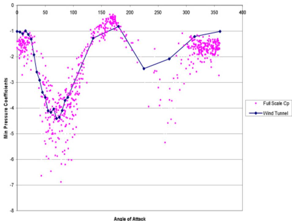
Fig. 3.3. Pressure coefficients measured at building corner, eave level, Texas Tech University experimental building (Long et al., 2006).
