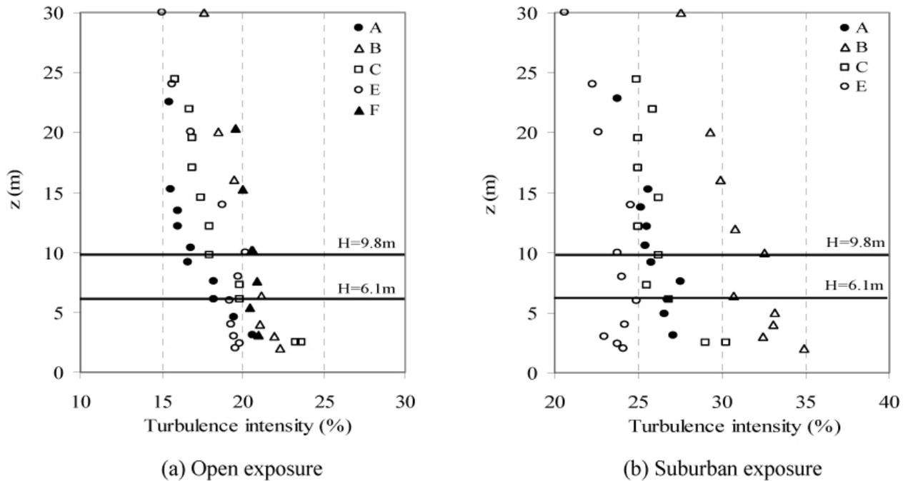
Figure 3.2. Turbulence intensities in simulations by wind tunnels participating in the Fritz et al. (2008) comparison (Bienkiewicz et al., 2009).
