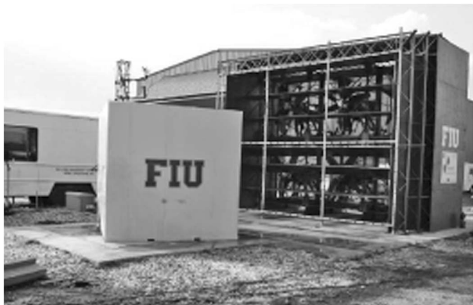
Fig. 2. 6-fan WoW and 2.9 m testing cube (image by A. Gan Chowdhury)
